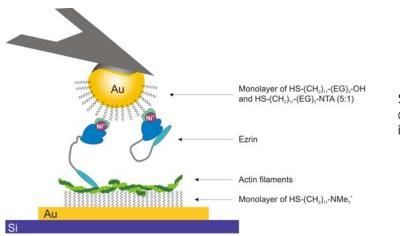
Schematics showing a colloidal sphere coated with ezrin for investigating interactions with F-actin.
