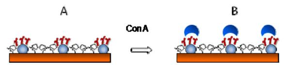
Binding of Concanavilin A (ConA) to surfaces functionalised with mannose clusters. A) Mannose biofunctionalised and PEG passivated gold nanostructured surface, and B) ConA bound to the mannosyl groups on the gold nanodots.
